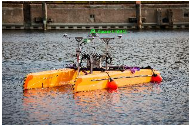
LiDAR (Ouster OS1) onboard SeaDragon USV
