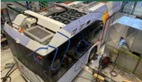
City Bus with Fuel Cell on Chassis Dynamometer
