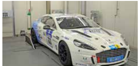
Racing Car with Bivalent (Hydrogen-Gasoline) Engine
