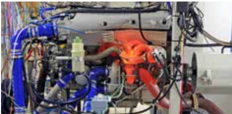
V12 Hydrogen Racing Engine on Test Bench
